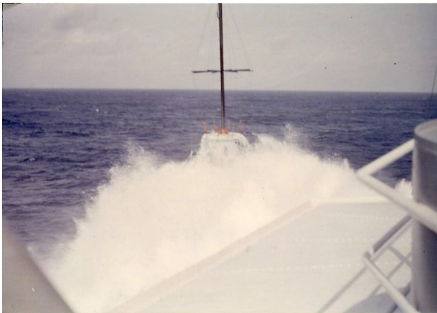
Figure 11 As the ship rises, the forecastle scoops up enough water to fill an Olympic size swimming pool. Photo from my personal collection.
