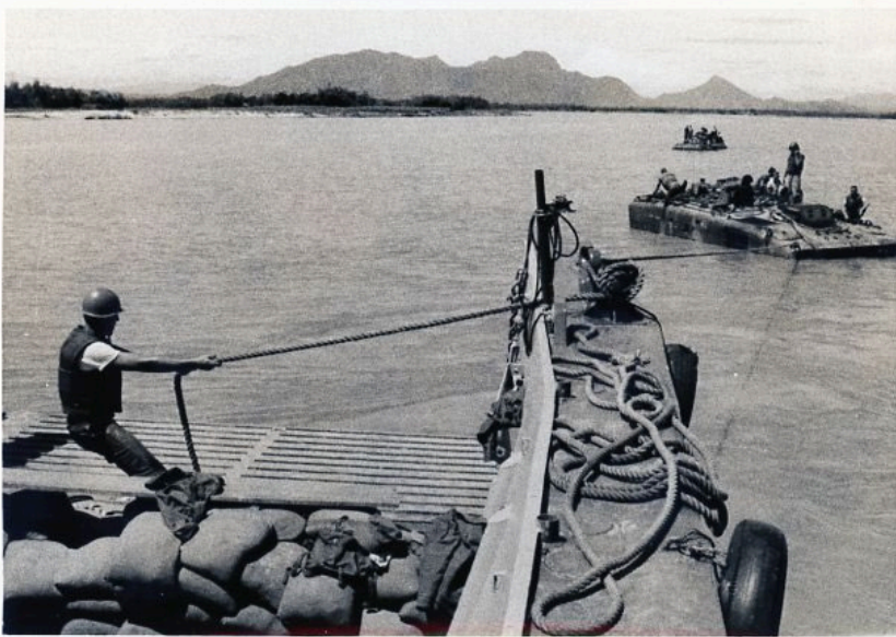
Figure 12 Quinn QM2 making a line fast on the 860s starboard cleat. The next step was to swing the boat to port, then swing rapidly back to starboard. The resulting force would jerk the 20-ton LVT out of the mud hole in which it was stuck.
